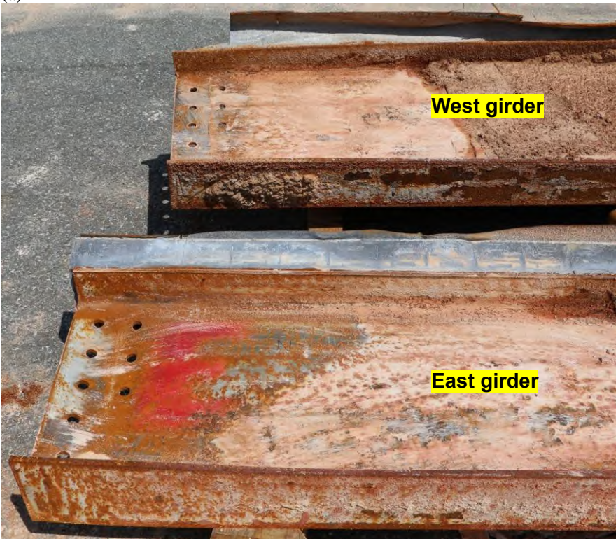
Fig. B-25. Post-test photographs of W18×35 girders in the test bay; (a) north end and (b) south end.
