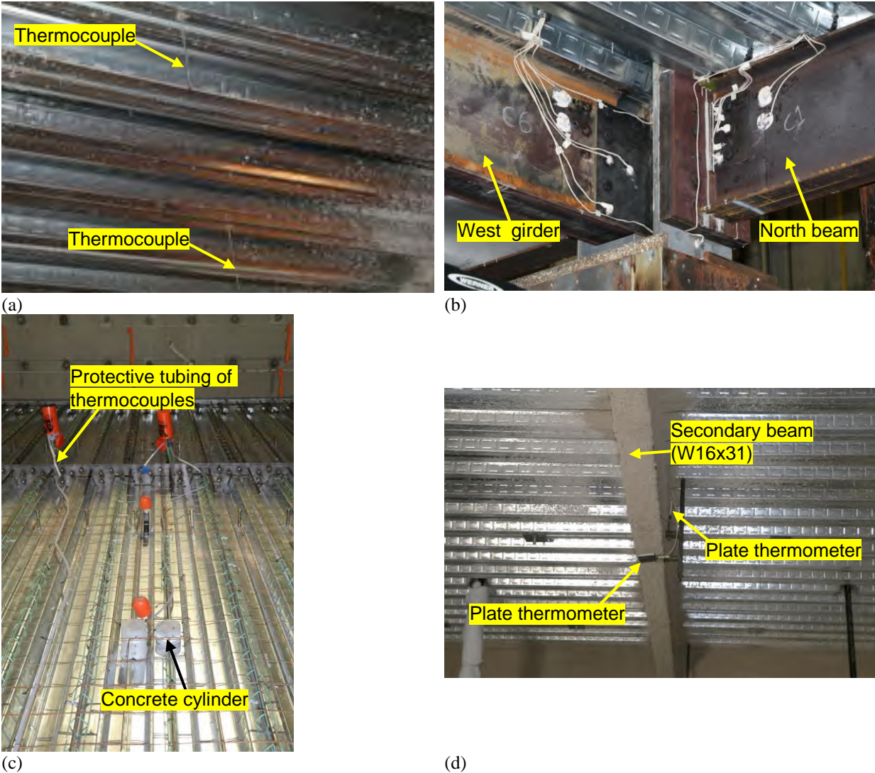
Fig. 3-4. Photographs of temperature sensors installed at (a) 305 mm below exposed steel deck; (b) ends of the west girder and the north beam prior to fireproofing; (c) top of the steel deck prior to concrete casting; (d) midspan of secondary beam.
